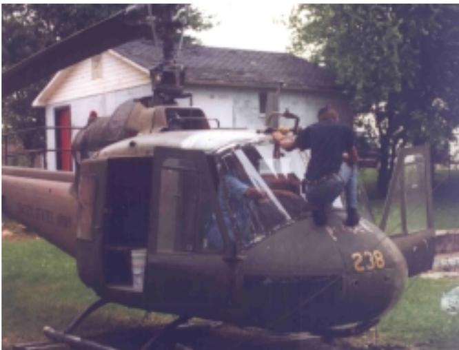
Windshields, both left and right hand to fill the void, took three sets of hands to install. Don Head peached on the nose for several hours while we installed the hundreds of nuts and bolts...
